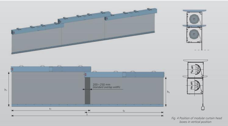
Fig. 3 Modular smoke curtain with vertical head boxes position
