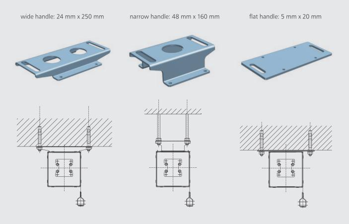
Thanks to the solutions used by Mercor, automatic mcr PROSMOKE curtains can be mounted to:
