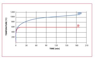
Diagram of temperature curve (D) and standard heating curve (DH)
