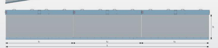
Fig. 5 Modular curtain in a linear system with a permissible gap at the curtain height of h > 2 m.
