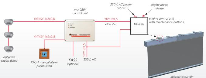
Fig. 11 Sample configuration of mcr PROSMOKE FS single curtain control system
