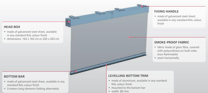
Smoke curtains are available with side guides (made of galvanised steel, in standard RAL colours), which can be used to create a sealed connection between the smoke curtain and the building structure for further reducing the smoke leakage
