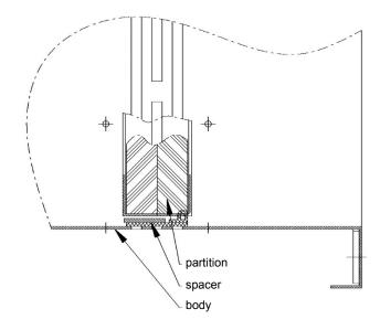
Securing the gap size between the damper body and the partition.
