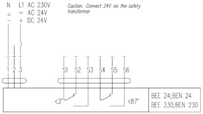
Several actuators can be connected parallely. Power intake should be controlled
