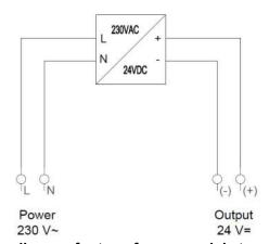
Connection diagram for transformer module type MP230/24
