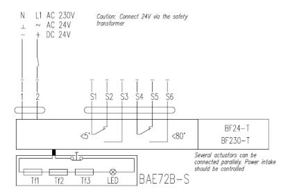
Connection diagram for the BF24-Tand BF230-T actuators
