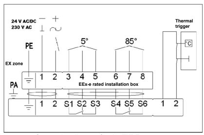
Connection diagram for the EXBF actuators
