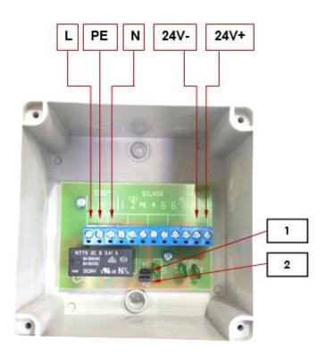
1. H1 jumper - removal releases the brake 24V - curtain descent
