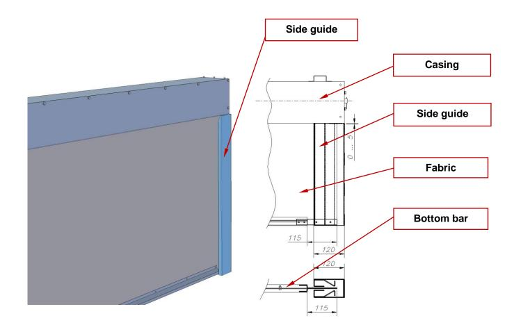
Fig. 22. Method of installing side guides
