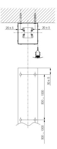
Fig. 8. Installation of a curtain without a suspension bracket
