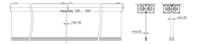
Fig. 16. Typical gap sizes in the transverse direction in the case of butt arrangement of curtain modules with type K, C and L casings and without fabrics overlapping
