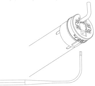
Fig. 6. Curtain limit switch adjustment
