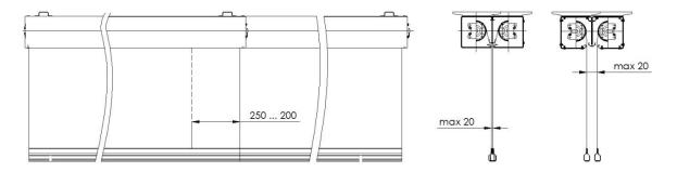
Fig. 15. Typical gap sizes in the transverse direction in the case of butt arrangement of curtain modules with type K, C and L casings and with fabrics overlapping
