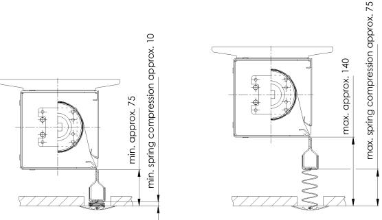
**Note**: Observe the minimum and maximum spring compression values. The distance between the casing and the ceiling is approximate.
