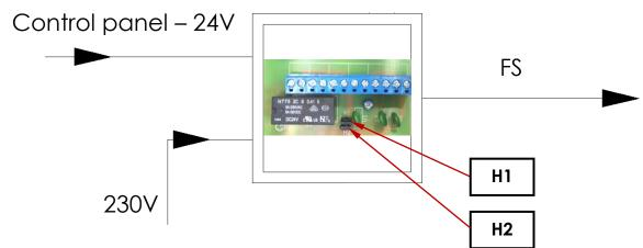
H1 – Removal of the jumper disconnects the brake
