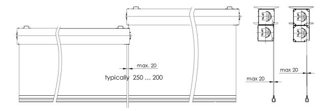
Fig. 14. Typical gap sizes in the transverse direction in the case of vertical arrangement of curtain modules without fabrics overlapping
