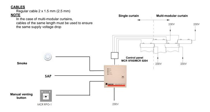
Fig. 10. Schematic diagram of the curtain connections with a common bottom bar
