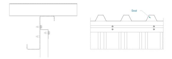
The spaces above the curtain should be sealed with mineral wool or cut-to-size sheet metal elements. Additionally, seal with fireproof foam, polyurethane Soudal Soudafoam 1K FR foam or a similar material.
