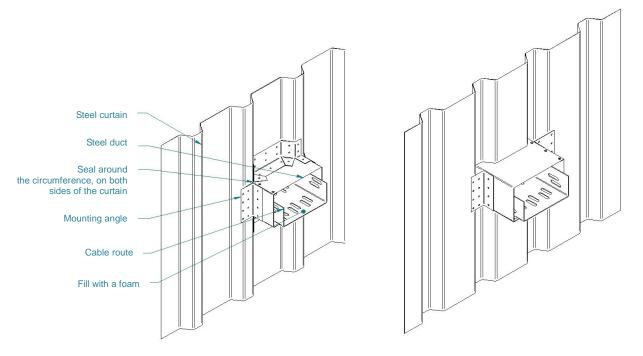
Example of an service penetration sleeve (view from both sides of the curtain)
