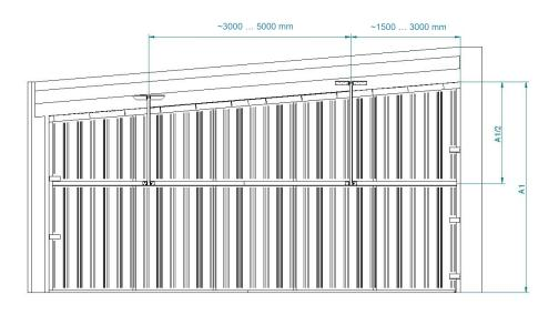
The reinforcements should be fixed in the middle of the curtain's height, at every  $3\div5$  m. Fix a steel angle to the curtain with self-drilling screws to the metal sheet. Fix the bracket to the angle and place the steel profile rotationally on the screw between them. At the other end, put the ceiling brackets on and fix them in the right place under the ceiling. Proceed in the same way with a steel cord (on both sides of the curtain).
