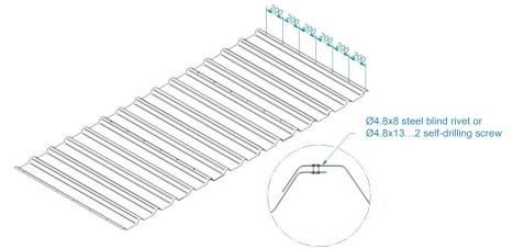
• Fix the covering profile at the bottom of the curtain with self-drilling screws for sheet metal.
