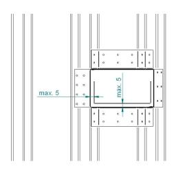
If it is necessary to pass an existing cable route through the curtain, the next trapezoidal sheets must be joined here (see section 5).
