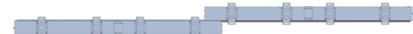
Fig. 17 Top view of mcr PROSMOKE FS/ CE modular smoke curtain in horizontal layout
